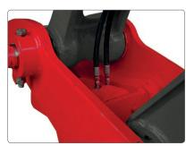
Simple and safe installation and operation comes from the need for only two hydraulic hoses to operate the both circuits of the coupler, and the solenoid valve which must be energized to release the attachment. This will ensure that in the event of an electrical failure the primary locking mechanism will stay in the locked position.
