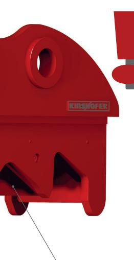
Greatest **SAFETY** due to separately controlled locking devices. The operator has to unlock the self-locking wedge as well as the  $X-LOCK^{TM}$  safety knuckle separately to change the attachment.
